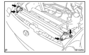
(c) Install the 2 radiator upper supports with the 4bolts. Torque: 12.5 N-m (128 kgf-cm, 9 ft-lbf)
