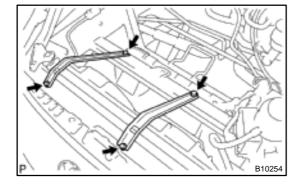
(f) Install the 2 spear wheel carrier extensions with the 2 bolts and 2 nuts.
